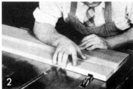
Blind dadoes in the cabinet sides are made on the circular saw with two 1/8" outside cutters and sufficient inside cutters to make a 3/4" wide dado.
