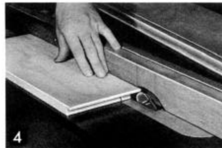
Finger mouldings on the drawer fronts are made on the circular saw with the No. 35-100 cutters mounted in the No. 265 moulding cutterhead. Note cut out auxiliary wood facing fastened to fence.
